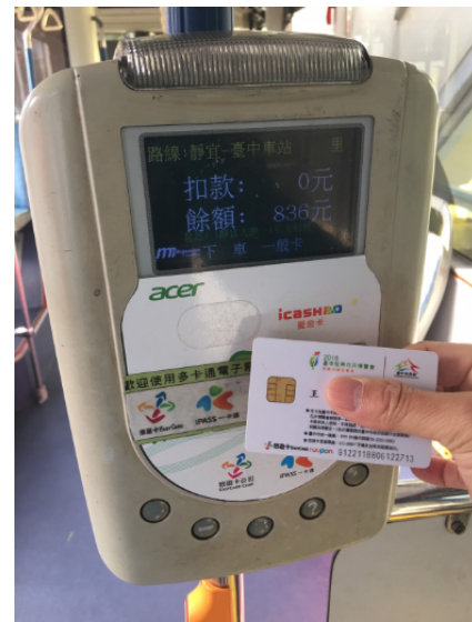
Fig. 4: A passenger should swipe his/her own card twice per trip when he/she gets on/off bus.
