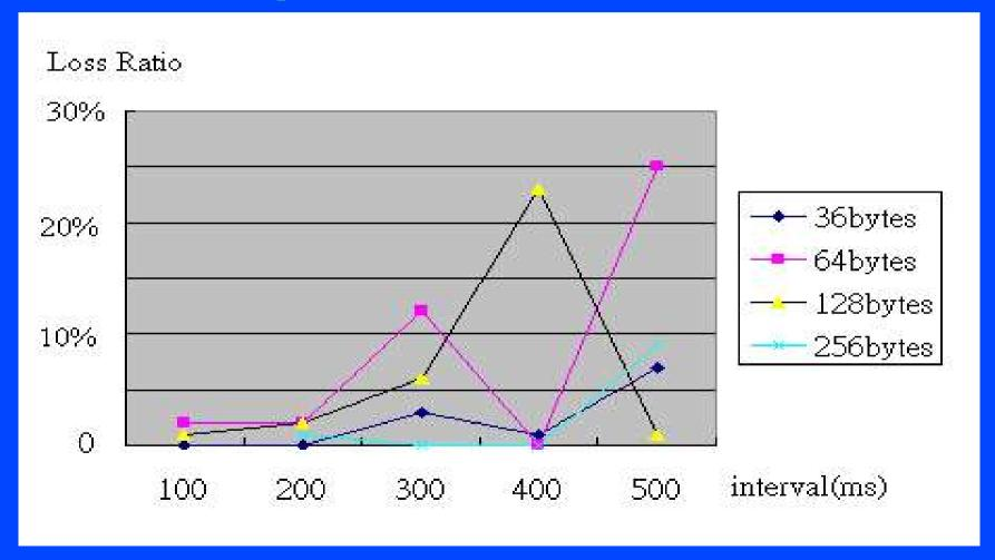
When transmission interval increase, packet loss ratio also increase.
