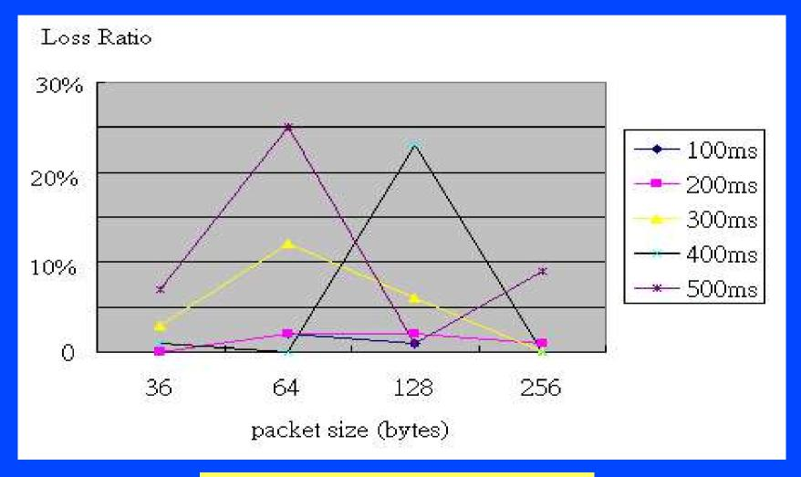
packet loss ratio is independent of packet size.
