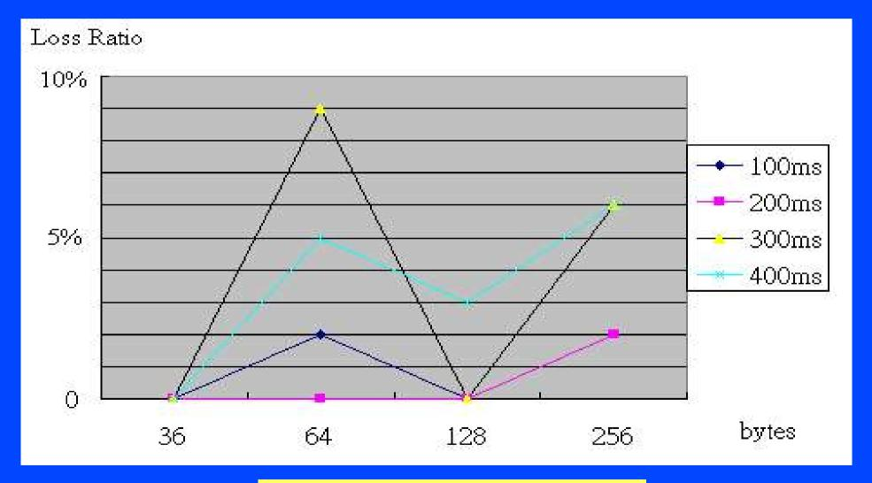
packet loss ratio is independent to packet size.
