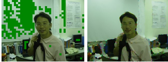
Fig. 6. (a) sum of AC^2 in green blocks < 100 (b) applying oil-paint effect selectively.
