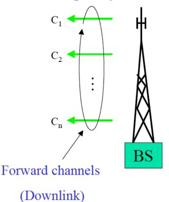
$C_i' \times C_j' = 0$ , i.e.,  $C_i'$  and  $C_j'$  are orthogonal codes  $C_i \times C_j = 0$ , i.e.,  $C_i$  and  $C_j$  are orthogonal codes
